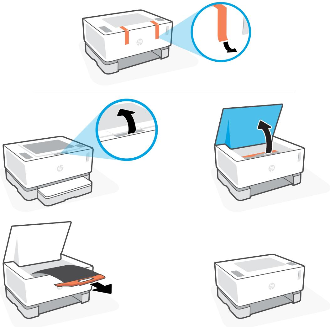
**EN** Remove the packing tape. Lift the top cover, and then remove and recycle the orange plastic handle with the attached black sheet.
