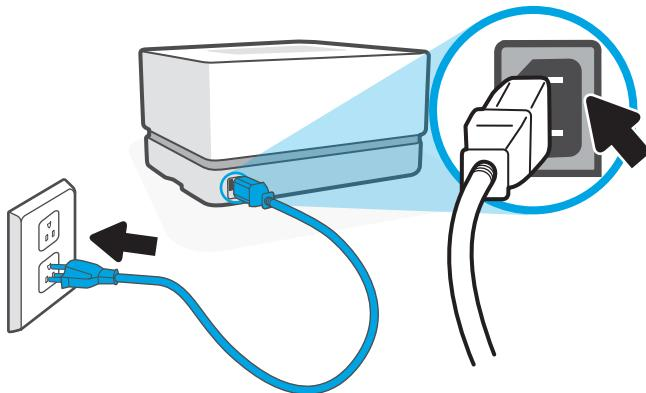
**EN** Plug in the printer. The printer turns on when it is plugged in and can take up to 1 minute to warm up. You will hear a series of noises, which is normal. When the Ready light
