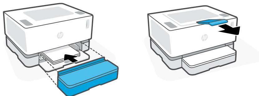
**EN** Install the input tray, load paper, and then slide the cover into place over the tray. Pull out the output bin extension.
