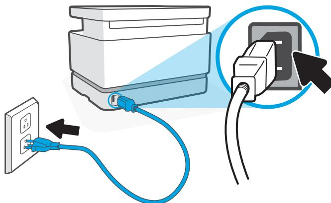
**EN** Plug in the printer. The printer turns on when it is plugged in and can take up to 1 minute to warm up. You will hear a series of noises, which is normal. When the Ready light
