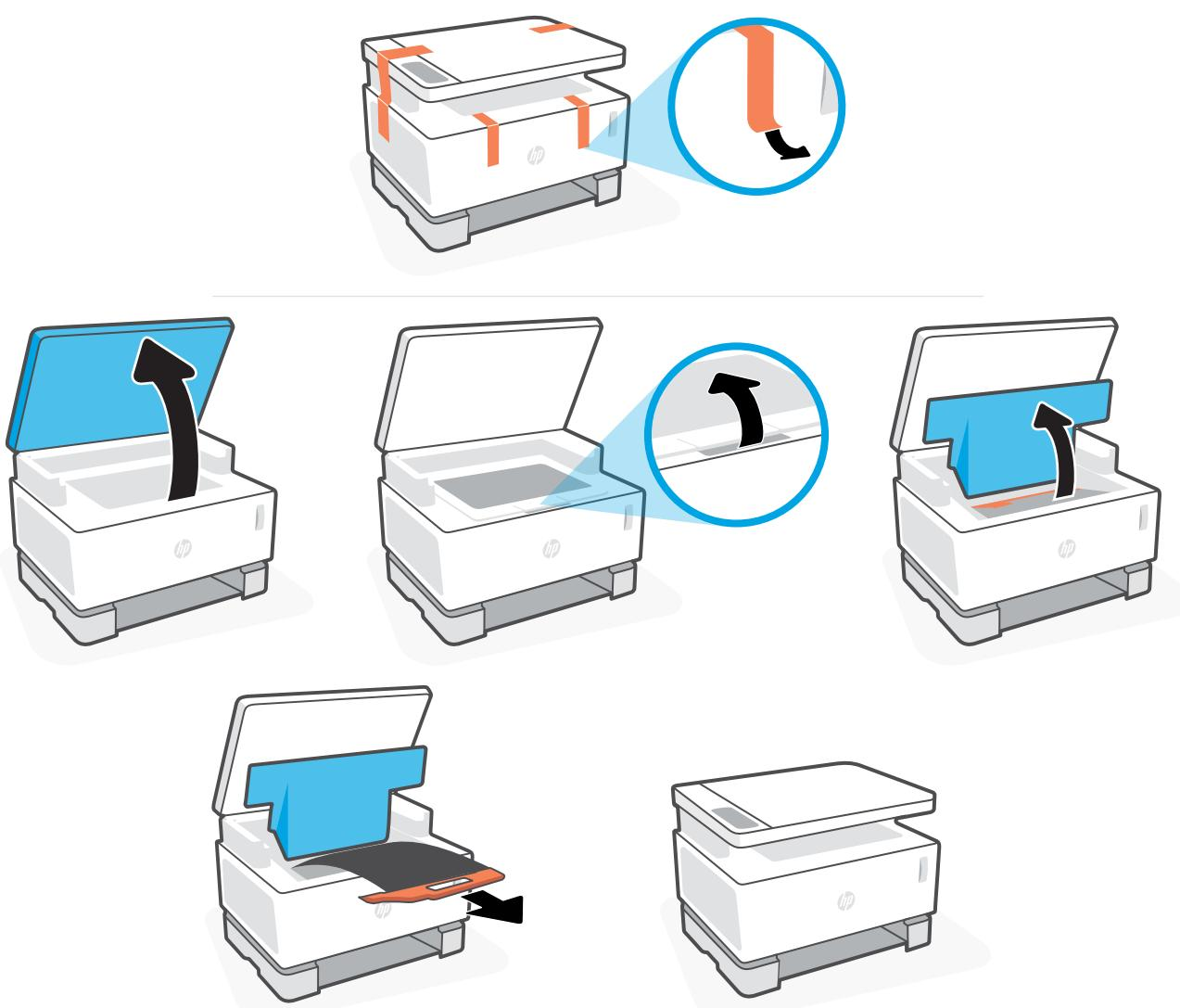
**EN** Remove the packing tape. Lift the scanner and the top cover. Remove and recycle the orange plastic handle with the attached black sheet.
