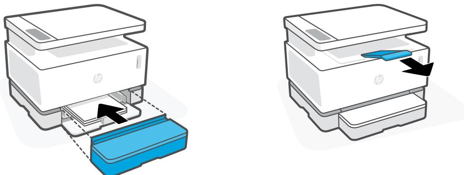
**EN** Install the input tray, load paper, and then slide the cover into place over the tray. Pull out the output bin extension.
